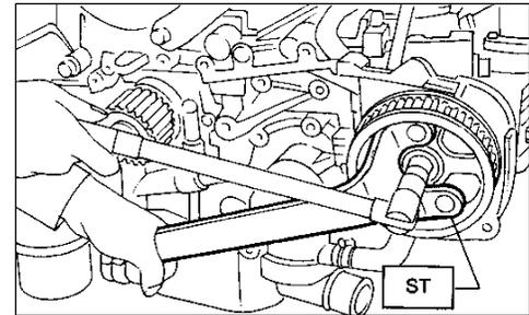
2. Remove the right side camshaft sprocket. To lock the camshaft, use ST 499207100 Camshaft Sprocket Wrench.
