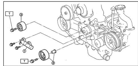
**Cautions:** *Do not allow pressure to exceed 9807 N (2205 lbs). Do not release the pressure until the stopper pin is completely inserted. Push the tension adjuster rod vertically. Press the push rod gradually, taking three minutes or more to fully retract the rod.*
