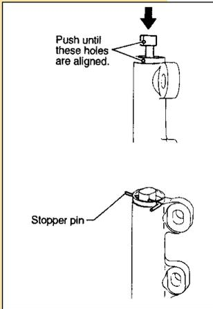
2. Install the belt tensioner and spacer.
