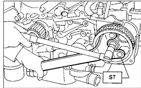
**Caution:** *Do not confuse the left and right side camshaft sprockets during installation. The left side camshaft sprocket can be identified by a projection used by the cam angle sensor to monitor camshaft position.*
